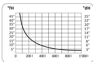
Volume of water filtered by the cartridge as a function of water hardness (°fH/°dH). See graph.
