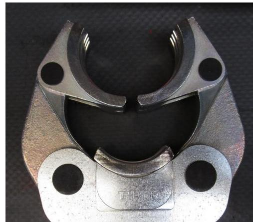
4.2. Place the crimping jaws on the fitting / pipe
