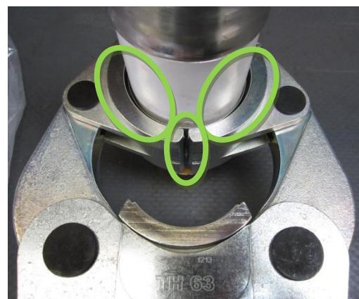
4.3. Slide the fitting / pipe to the fixed groove of the crimping jaws.
